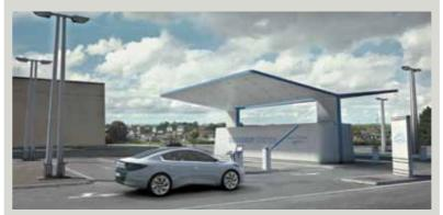
3. 3-minute Quick Drop battery exchange system: at specially-equipped stations, a machine swaps the used battery for another without the driver even having to leave the vehicle. Exclusive to Renault-Better Place.
