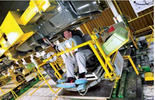
Sovab Batilly - Mastics workshop- underbody tool trolley for person of reduced mobility. Pedal or joystick control.
